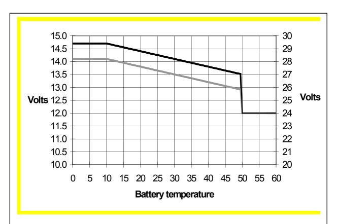
Default output voltages for Float and Absorption are at 20°C. Reduced Float voltage follows Float voltage and Raised Absorption voltage follows Absorption voltage. In adjust mode temperature compensation does not apply.
