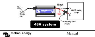
Minimum battery capacity should be 20Ah. Make sure you connect the RED wire to the positive (+) terminal of the battery and the BLACK wire to the negative (-) terminal.
