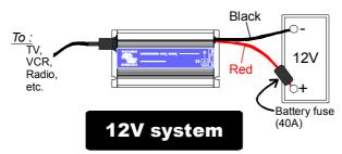
Minimum battery capacity should be 50Ah. Make sure you connect the RED wire to the positive (+) terminal of the battery and the BLACK wire to the negative (-) terminal.
