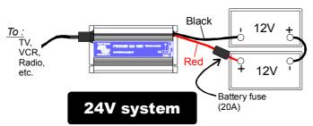
Minimum battery capacity should be 30Ah. Make sure you connect the RED wire to the positive (+) terminal of the battery and the BLACK wire to the negative (-) terminal.
