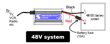
Minimum battery capacity should be 20Ah. Make sure you connect the RED wire to the positive (+) terminal of the battery and the BLACK wire to the negative (-) terminal.
