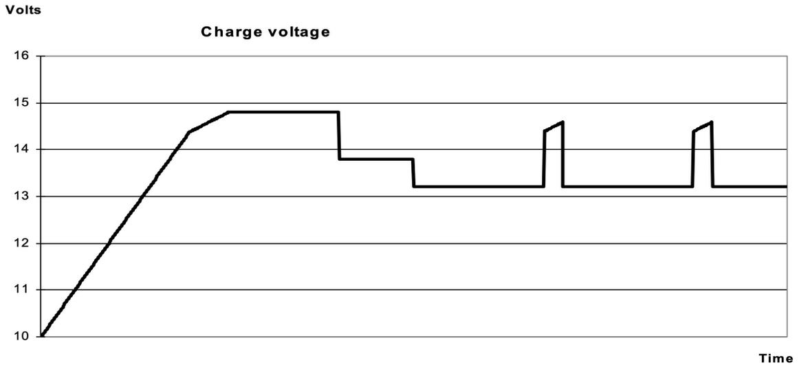
**i** The voltages in the above table are for a 12V battery bank. To arrive at 48V battery bank voltages, multiply the 12V voltages by a factor of four.
