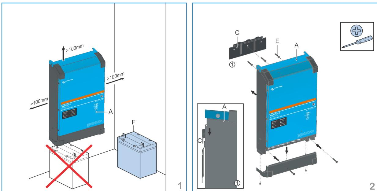
Refer to the [Dimensions \[41\]](#) chapter for the location and dimensions of the mounting holes.
