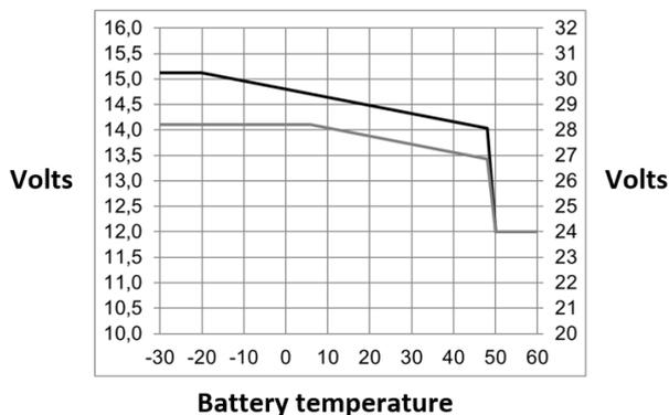
Default output voltages for Float and Absorption are at 25 °C for 12 or 24V battery bank.
