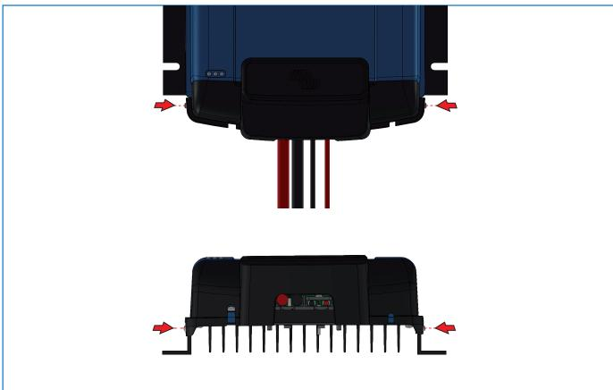
STEP 3: Place the WireBox cover and fasten with two screws.
