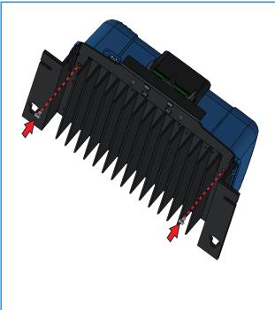
STEP 1: Mount the 'steel base' to the MPPT before installation to the wall.
